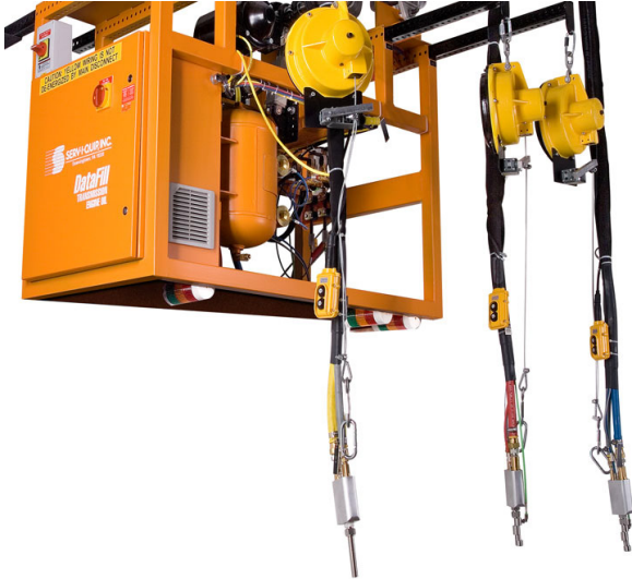
DataFill Transmission, Engine Oil, & Differential Fill System with VF Drive
